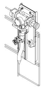
5. Mount the KP1H system to the extension plate using the 4 screws supplied in the kit.
