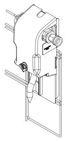
Rout the pick up tubes thru the openings in the extension plate. Attach them to the Dial-4 valve and replace the cover.
