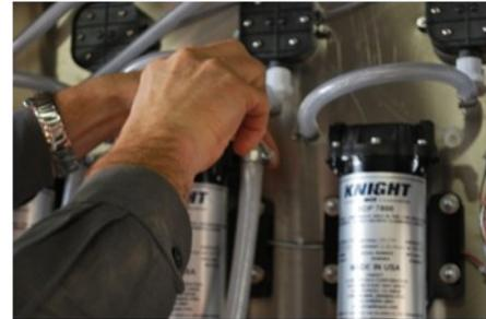
**Note: Maximum suction hose length is 10 ft (3.04 M) between pump and bottom of chemical concentrate tank.**
