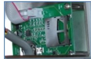
**The Input-Output Board** connects all the pumps, flow meters, floats, and temperature probe to the Main Controller. When the Main Controller issues a command to the Input-Output board to blend the teat dip, the pumps and flow meters, sensors and probes work together to blend a superior quality teat dip.
