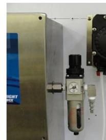
**Installation Space:** The DAIRY CHEM PLUS systems are designed for wall mounting. Make sure the wall surface is flat enough to allow flow meters to orientate at 90 degrees to the floor.
