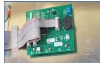
**The Memory Module** links directly to the Main Controller and collects all of the chemical blending event data for managing quality of the chemistry produced, monitoring consumption and invoicing the customer according to the teat dip produced. An integrated SD type (media card) reader provides a simple means of downloading report files and uploading settings to the system.
