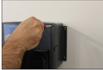
(14) Loosen two cover screws.
