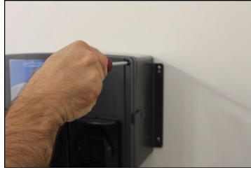
(14) Loosen two cover screws.
