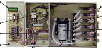
Lube zone valves with external tubing connectors
