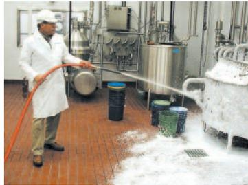
The dryness or wetness of the foam can be adjusted for different cleaning applications with a simple turn of a knob.
