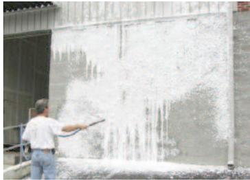
FoamClean foamers have a higher and longer throw than competitors with a projection distance of 30 feet (9 meters).
