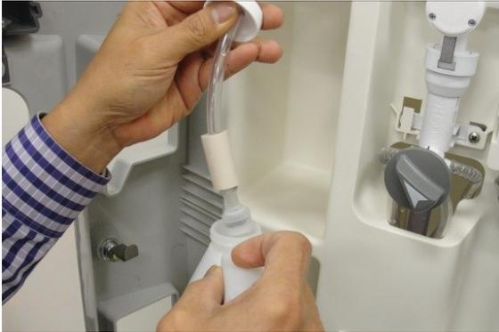
**Step 10.** Connect bottle caps onto the chemical containers. Place containers into cabinet.
