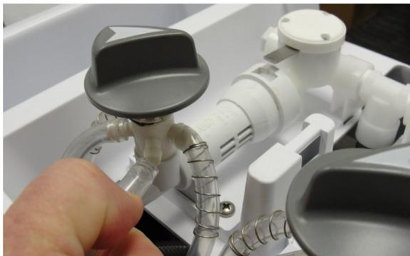
**Step 7.** Remove one of the chemical lines from the port it is attached to in preparation for installing a metering tip.
