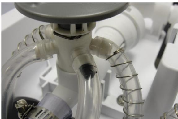
**Step 9.** Re-connect chemical line over the metering tip and cinch a plastic tie around the barb to secure it. Repeat for all other ports on the unit
