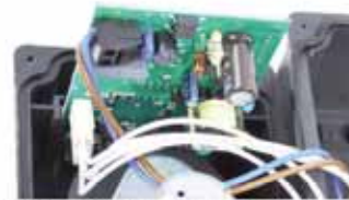
Plugs on the circuit board provide for quick electrical connection
